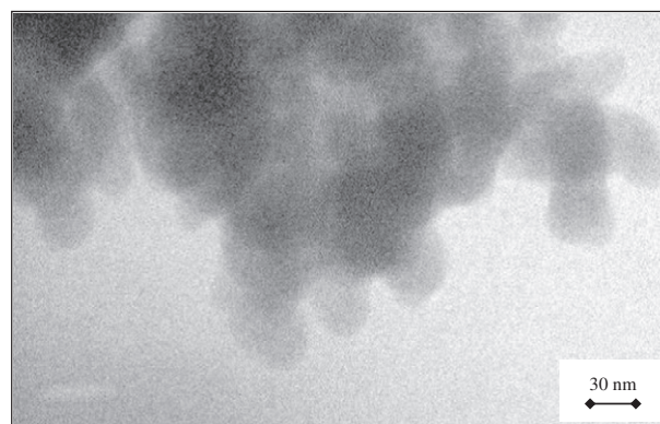
Fig. 2. TEM image of a typical sample of colloidal CdS:Mn nanocrystals.
