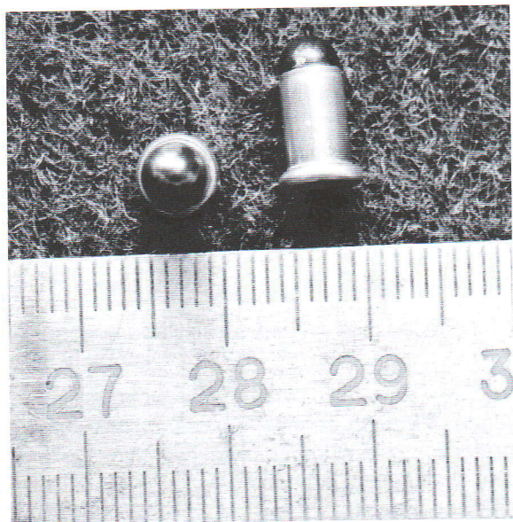
Fig. 1. Cartridge of the bullet of Flaubert type "4 mm long"
